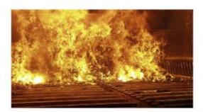
Confined and controlled burning, known as combustion, can not only decrease the volume of solid waste destined for landfills but can recover energy from the wasteburning process to generate electricity. A moving grate incinerator is capable handling 15 tons of waste per hour. This generates an energy reduces carbon and emissions by offsetting the need for energy from fossil sources reduces and methane generation from landfills.
